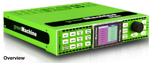
The current greenMachine titan comprises four 3G/HD/SD-SDI video channels or a single 4K/UHD video channel. It offers up to 12G processing support (3840 x 2160 @60 Hz) and provides the functionality to convert between single-link 4K video (12G) and quad-link 4K video (2SI; 4x3G).
