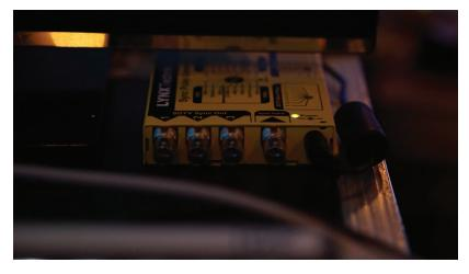
The whole SDI broadcast setup was synchronized to the master clock generated by the yellobrik HD / SD Sync Pulse Generators with Genlock.
