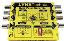
The SPG 1707 is portable sync generator that includes genlock with full cross lock capability, which locks the outputs to any reference sync format and standard. The module provides 3 x HDTV tri-level sync outputs as well as 3 x SDTV bi-level sync outputs and supports all SD, HD and composite (PAL / NTSC) video formats. A separate audio sync output can be switched between 48 KHz Word Clock or Digital Audio Reference (DARS).
