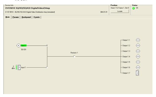
The input detection indicates the bit rate (SD-SDI = 270MBit/s, HD-SDI = 1.5 GBit/S; 3G-SDI = 3GBit/s) of a connected signal. If no signal is detected the color of the input detection will turn red.
