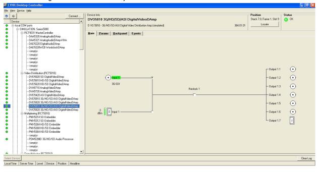
The above screenshot shows the complete module GUI. The Device info area contains information about the module including name and firmware revision. If used as part of a larger system (using the LYNX central control system) the modules position and physical location is displayed above the "locate" button.
