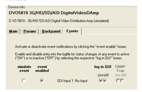
The GUI has an integrated error log, which is a simple text log file stored in the controller PC. This will record an event and timestamp it. The log can be seen at the bottom of the GUI screen and can be scrolled through using the scrolling bar.
