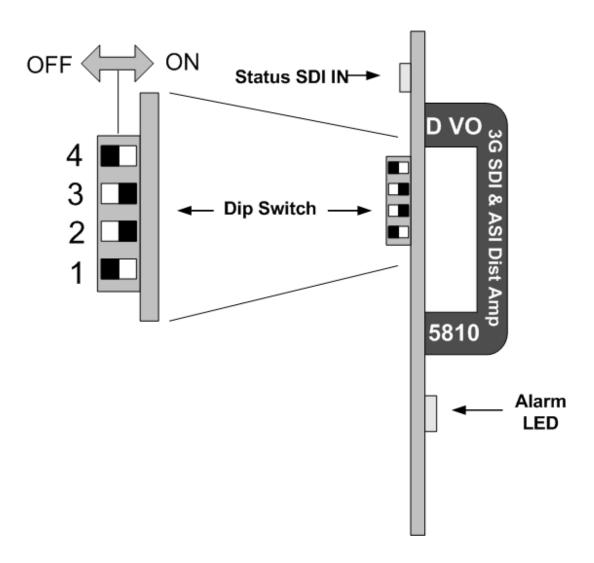
Figure 3 – Switch and LED locations
