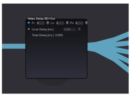
The output delay can be adjusted for the SDI output either in frames, lines and pixels or in ms. The total delay can be up to 62 frames.
