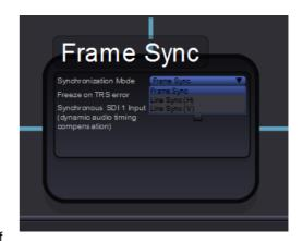
the input signal to the Frame Pulse of the Reference. This results in frame aligned signals without the additional 1 frame delay of the frame synchronizer mode.
