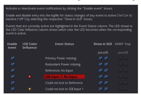
The GUI has an integrated event log, which is a simple text log file stored in the controller PC. This will record an event and timestamp it. The log can be seen at the bottom of the GUI screen and can be scrolled through using the scrolling bar.
