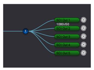
Double Clicking on the small (blue) bubble with the "t" inside will show the timing adjustments for the SDI outputs as shown below.
