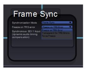
"Timing Reference Signals" and is a sequence of digital values embedded in the SDI data streams. If the frame synchronizer cannot recover these errors, then the channel will freeze the video until the errors can be recovered. One function of the synchronizer is to repair any bad TRS values ensuring a stable and technically correct video stream is delivered on the outputs. Selections for each channel are as follows:
