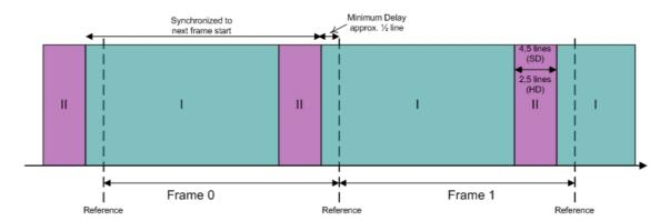
For distortion free switching in front of the P VD 5802, e.g. in a router, all signals have to be in area "I" or all signals in area "II".
