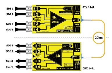
The fiber connection is made between each **COM** port. The UPG port is used to connect the OTR 1442 to add 4 more SDI channels.
